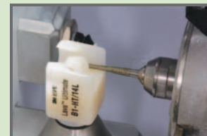
The TS150 mill producing a restoration from a block of Lava Ultimate
